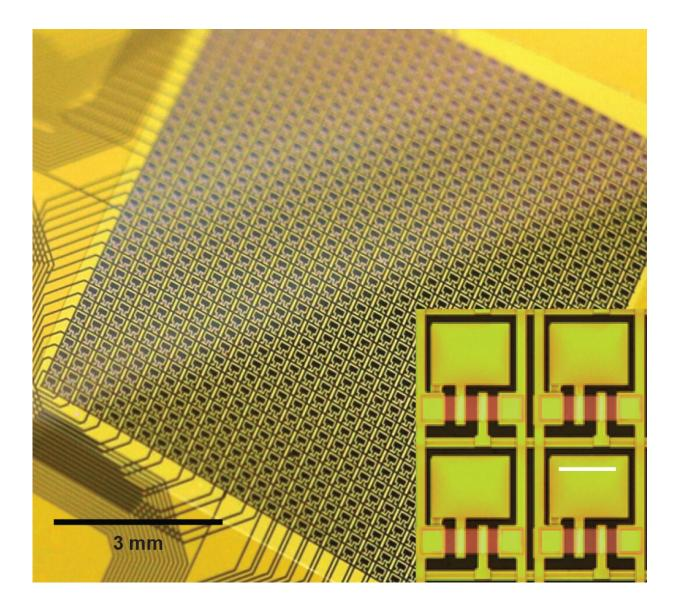
A photograph of the Neural Matrix array, which allows for high-resolution and long-term microelectrocorticography. Credit: C.-H. Chiang et al., Science Translational Medicine (2020)
