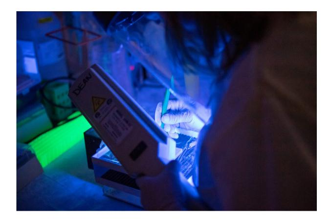
Working with ultraviolet light, Vilander removes DNA bands from agarose gel following electrophoresis. The steps are a move toward constructing an experimental vaccine against coronavirus. Credit: John Eisele
