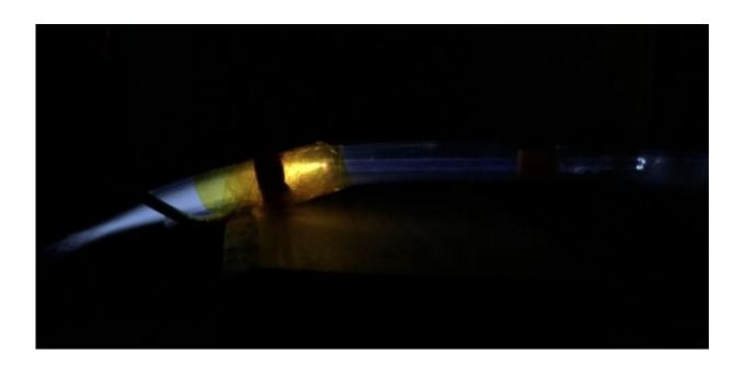
Image of a plasma plume generated from flowing argon in a plastic tube. Room-temperature plasma creates reactive oxygen and nitrogen species during interactions with ambient air. Credit: Sean Knecht
