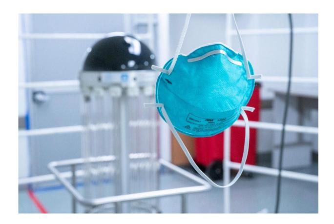
When the machine is operating, the racks surrounding it are fully loaded with masks for sanitizing. Tru-D can disinfect hundreds of masks per each 20-minute cycle. Credit: Sanjay Suchak, University Communications
