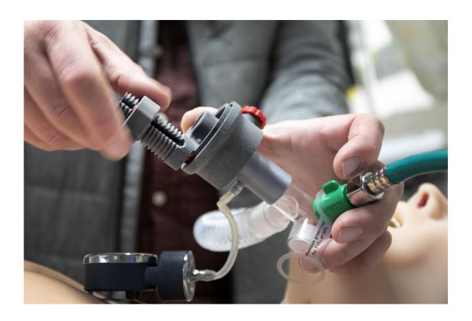
The ventilator design does not require electricity and operates off of a standard oxygen tank. Credit: OHSU/Kristyna Wentz-Graff
