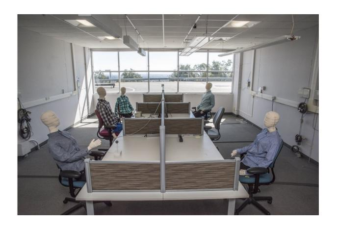
FLEXLAB(R), the world's most advanced building simulator and testbed, will be used to simulate office and school heating, ventilation, and air conditioning configurations. Credit: Berkeley Lab
