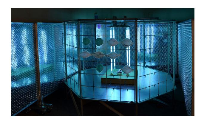
The device's targeted capacity is approximately 3,000 N95 masks per day (200 masks per exposure), but St. Luke's can scale up to 10,000 masks per day if necessary. Credit: St. Luke's University Health Network
