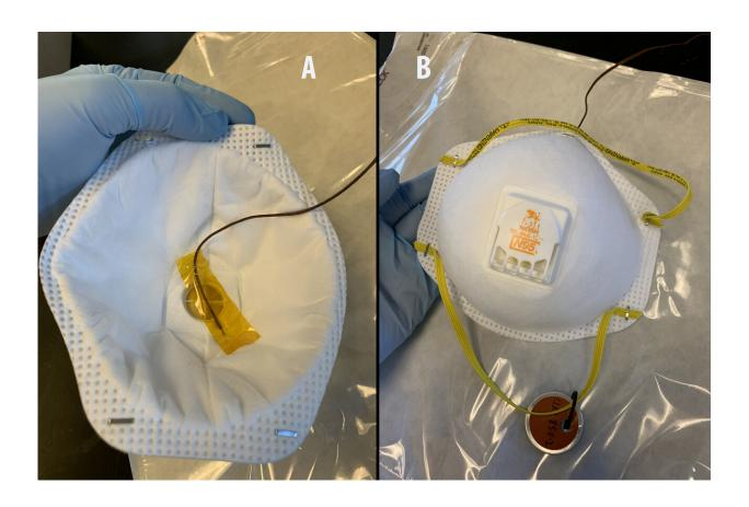
Inner and outer view of an N95 mask between dry heat treatment cycles showing no deformation of the respirator. A thermocouple is affixed to the inner surface of the respirator with Kapton tape to measure the surface temperature of the mask over 10 heating cycles in a standard laboratory convection box oven. Masks are heat treated inside a self-sealing autoclave pouch (background) to prevent dispersion of viral particles from airflow inside the oven. Credit: Trevis Massey/LLNL
