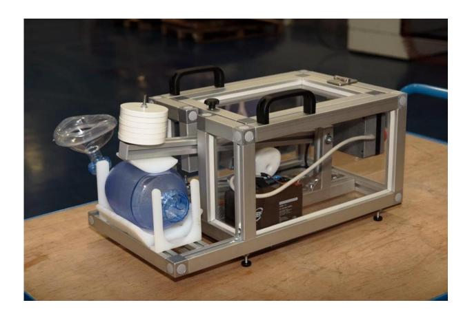
Realized by researchers at Istituto Italiano di Tecnologia and University of Ferrara, DIEGO is an innovative engineering solution composed by a respiratory bag (Ambu-like) coupled with an electric motor which manoeuvres a lever. Its simple design makes the device to be easily replicable and quickly available to be used in an emergency scenario where it is difficult to purchase new medical instruments. Credit: IIT-UniFe
