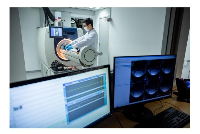
The team carries out experiments on mice using the 3T MRI animal scanner at CityU, the only of its kind in Hong Kong. The left computer screen in the front shows vital signs such as the pulse and breathing pattern of the mouse, while the right one shows the images of its brain. Credit: City University of Hong Kong
