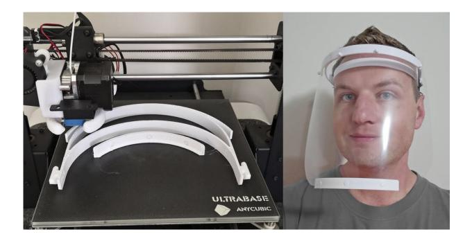
A Prusa RC3 face shield 3-D printed on a desktop 3-D printer. Credit: James Novak
