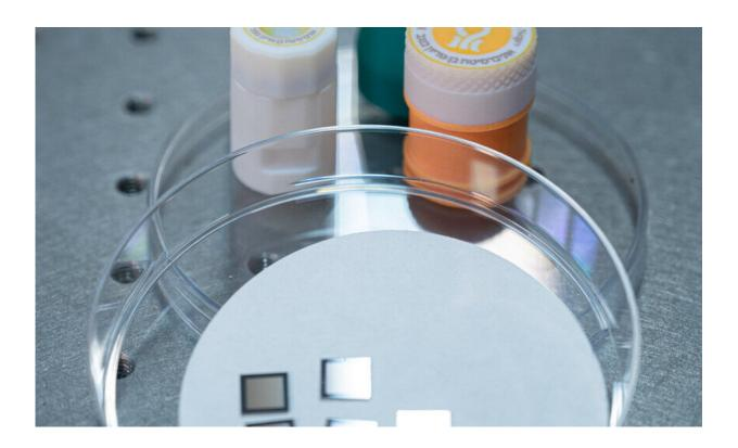
Particles from a simple breath test or throat and nose swabs, currently used for other tests, are placed on a chip with a dense array of tens of thousands of metamaterial sensors that were designed specifically for this purpose. The system then analyzes the biological sample and provides an accurate
