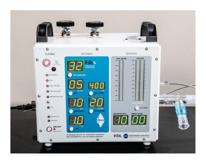
VITAL (Ventilator Intervention Technology Accessible Locally) is a new high-pressure ventilator developed by NASA and tailored to treat coronavirus (COVID-19) patients. Engineers at NASA's Jet Propulsion Laboratory in Southern California designed the device to free up the nation's limited supply of traditional ventilators so they may be used on patients with the most severe
