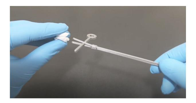
The testing swab is comprised of PLA-printed plastic and a folded and wrapped rayon sheet. Credit: NJIT
