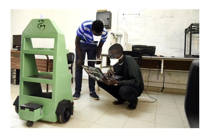
The robot dubbed "Dr. Car" should be able to measure blood pressure and temperature, reducing exposure to infected patients and the use of expensive protective clothing
