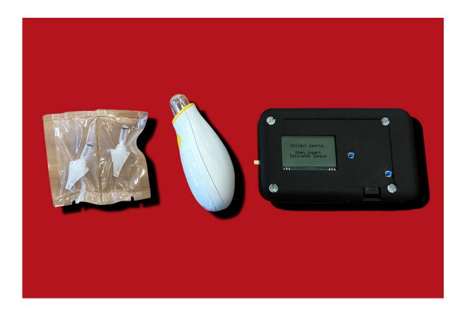
Ming Wang, distinguished professor of civil and environmental engineering at Northeastern, developed a testing device to monitor glucose levels using rapid saliva samples. The device, he says, can be tweaked to test for COVID-19. Credit: Matthew Modoono/Northeastern University
