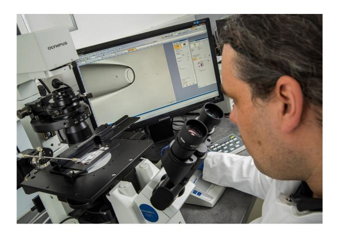
Under the microscope, Bernhard Polzer isolates single cancer cells he previously obtained from patient material. The monitor shows the glass capillary with the cell he previously identified as a cancer cell and then suctioned off the slide. Credit: Fraunhofer ITEM/P. Reinig
