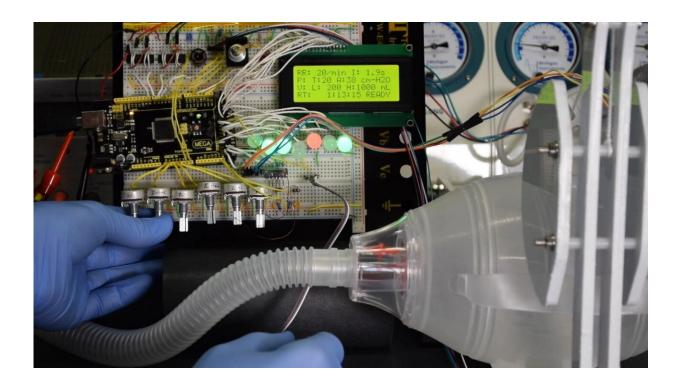
The ventilator is controlled by pressure sensors, rather than volume sensors, which allowed researchers to lower the device's price dramatically. Credit: University of California San Diego
