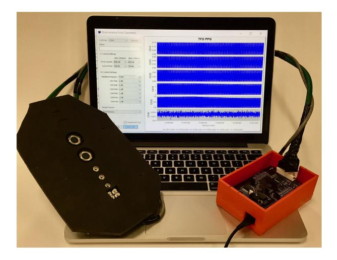
Prototype of the external fetal oxygen monitor developed by engineers at UC Davis. The device uses light to directly measure fetal oxygen saturation. Existing monitors used in the delivery room infer fetal oxygen by measuring fetal heart rate and contractions, and have a high false positive rate leading to many Cesarean sections. The new device has so far been successfully tested in sheep. Credit: Daniel Fong, UC Davis
