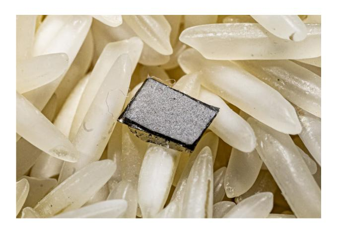
A sample of Rice University's 'magnetoelectric' film atop a bed of uncooked rice. Rice neuroengineers created the bi-layered film to power implantable neural stimulators that are approximately the size of a grain of rice. The film converts energy from a magnetic field directly into an electrical voltage, eliminating the need for a battery or wired power connection. Credit: Jeff Fitlow/Rice University
