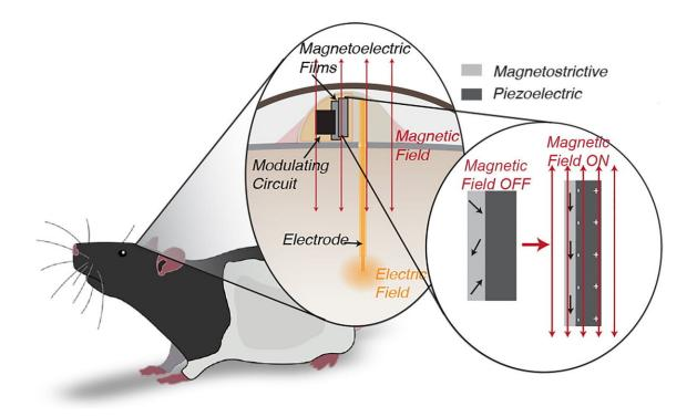
To demonstrate the viability of miniature, magnetoelectric-powered neural stimulating technology, Rice University neuroengineers created tiny devices that were placed beneath the skin of rodents that were free to roam throughout their enclosures. The rodents preferred to be in portions of the enclosures where a magnetic field activated the stimulator and provided a small voltage to the reward center of their brains. Credit: J. Robinson/Rice University
