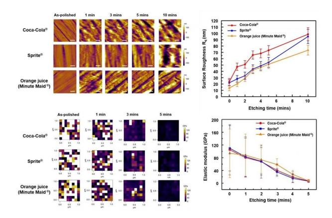
Changes in surface roughness (top) and modulus of elasticity (bottom) of tooth enamel exposed to popular beverages imaged by atomic force microscopy.
