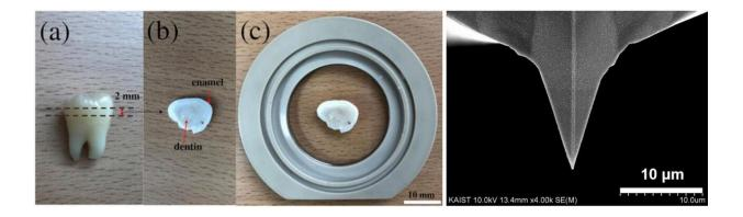
Tooth sample preparation process for atomic force microscopy (a, b, c), and an atomic force microscopy probe image (right). Credit: Professor Seungbum Hong, KAIST
