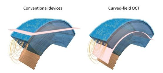
Traditional imaging approaches acquire a flat slice (pink) that crosses through several corneal layers at once, limiting the field of view (left). The new curvedfield OCT approach matches the curvature of the cornea to provide a larger imaging area (right). Credit: Viacheslav Mazlin, The Langevin Institute
