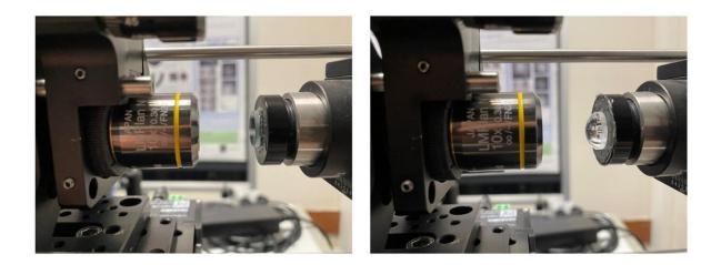
To capture images from a curved sample, such as a cornea, the researchers replaced the flat mirror (left) of a traditional full-field OCT setup with a curved optical lens (right). The curved lens optically flattens the acquired images. Credit: Viacheslav Mazlin, The Langevin Institute
