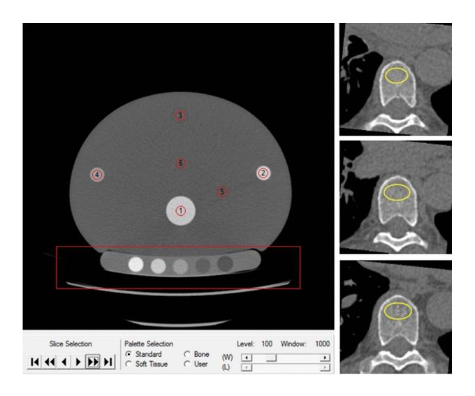
The Mindways Solid phantom with volume of interest in the quality assurance phantom (red circles, left side). A participant's noncontrast-enhanced axial CT (right side) with volume of interest (yellow circles) in the trabecular bone compartment of three vertebrae for bone mineral density measurements. Credit: Radiological Society of North America
