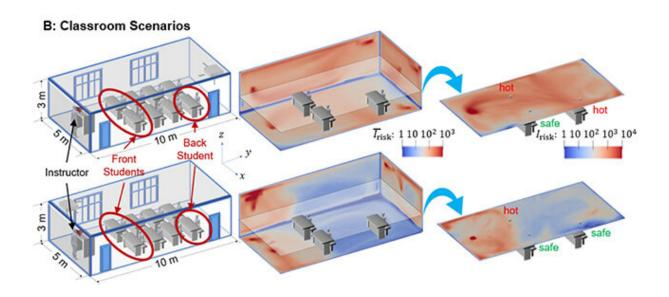
A numerical simulation shows aerosol transport and deposition in a small classroom setting with an asymptomatic instructor and the ceiling ventilation system located in the back (top) and front (bottom) of the classroom. Credit: Suo Yang, University of Minnesota
