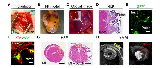
In vivo implantation and long-term evaluation of 4D patches. (A) Optical image of surgical implantation of the patch. (B) Optical image of a heart I/R MI model
