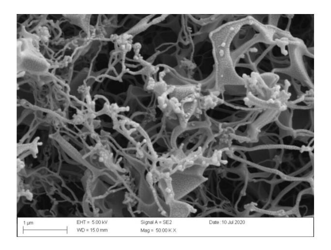
A microscopic image of remdesivir powder formulations after the thin-film freezing process. All formulations exhibited a brittle matrix structure of highly porous particles. Credit: University of Texas at Austin
