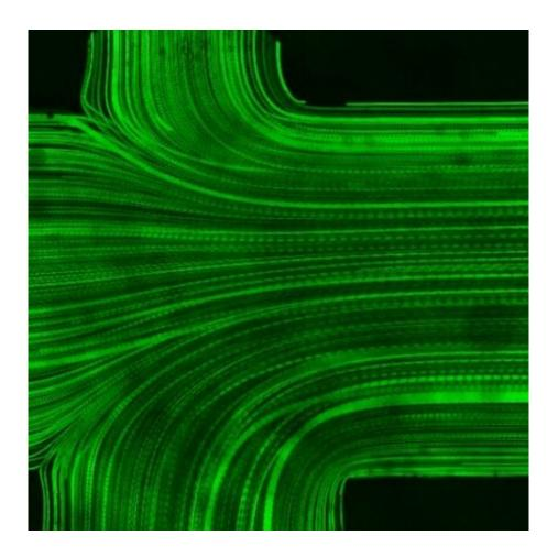
This is a time-lapse microscopic image of particle-based flow visualization inside a ventricular catheter. The image shows the confluence of three flows: the upstream flow coming from the catheter tip direction and two flows coming in via holes facing each other. Credit: Bourouiba Research Group
