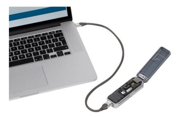
Oxford Nanopore Technologies' MinION is a palm-size DNA sequencer. Credit: Oxford Nanopore Technologies
