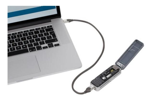
Oxford Nanopore Technologies' MinION is a palm-size DNA sequencer. Credit: Oxford Nanopore Technologies
