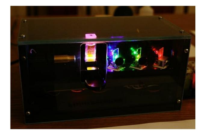
Laser-induced fluorescence is a method of using lasers to cause specific substances to emit light. Credit: Jan Pavelka/Wikimedia Commons, CC BY-SA
