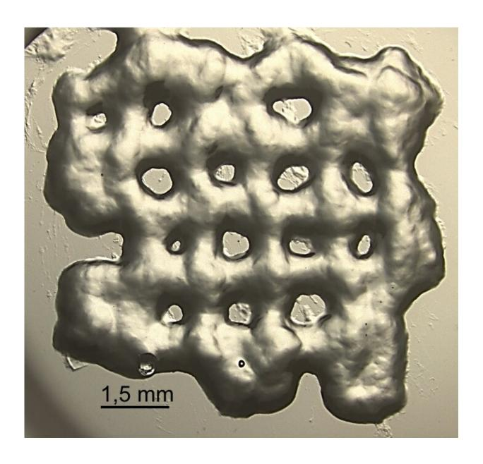
Initial prototype of a hydrogel scaffold manufactured with a 3-D printer. Credit:
