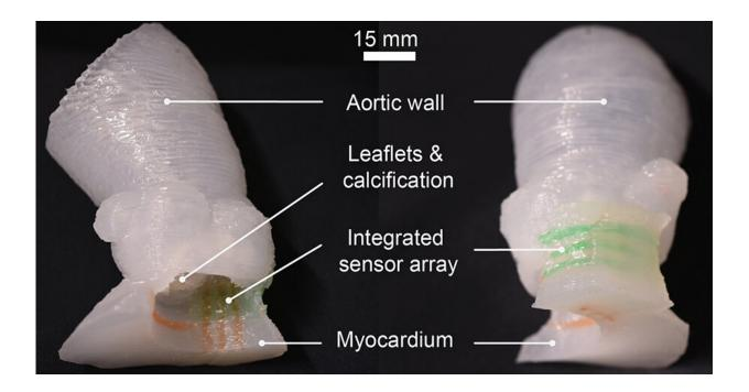
Patient-specific organ models, which include integrated 3D-printed soft sensor arrays, are fabricated using specialized inks and a customized 3D printing process. Such models can be used in preparation for minimally invasive procedures to improve outcomes in thousands of patients worldwide. Credit: McAlpine Group, University of Minnesota
