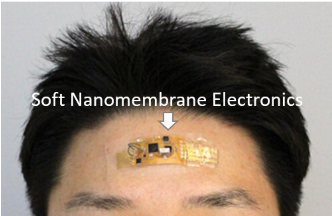
The wearable sleep monitoring device developed by W. Hong Yeo
