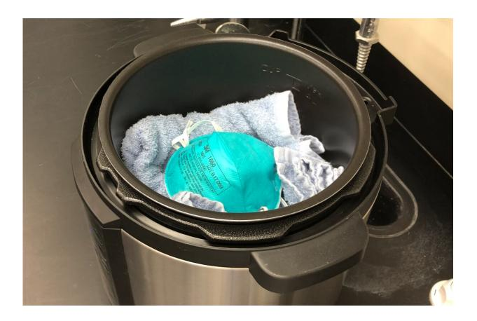
A towel keeps the respirator from touching the heating element on the bottom of the cooker. Credit: Chamteut Oh
