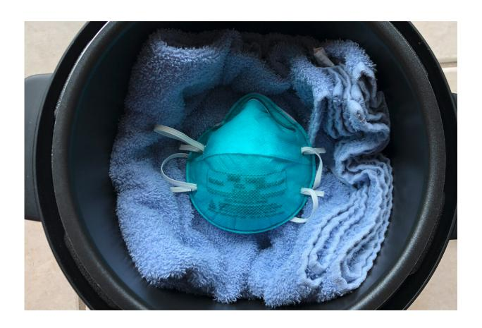
One 50-minute, 212 F cooking cycle in a dry electric multicooker decontaminates an N95 respirator without chemicals and without compromising the filtration or fit. Credit: Chamteut Oh
