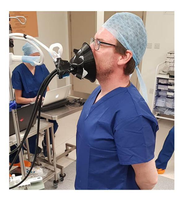
Scientific experiment to measure the spread of aerosols emitted when singing is conducted in an orthopaedic operating theatre, an environment of "zero aerosol
