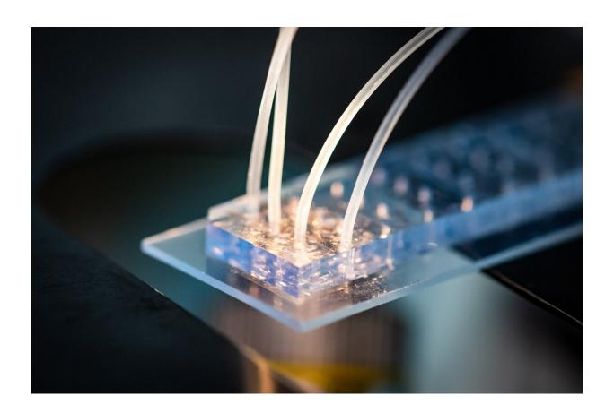
Magnification of miniature chips: Single cells are encapsulated in tiny droplets and supplied with reagents for further processing. Credit: Felix Petermann, MDC
