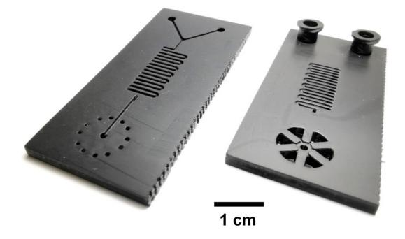
Illinois researchers developed a microfluidic cartridge for a 30-minute COVID-19 test. The cartridges are 3D-printed and could be manufactured quickly. Credit: Bill King, University of Illinois
