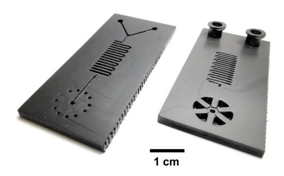
Illinois researchers developed a microfluidic cartridge for a 30-minute COVID-19 test. The cartridges are 3D-printed and could be manufactured quickly. Credit: Bill King, University of Illinois
