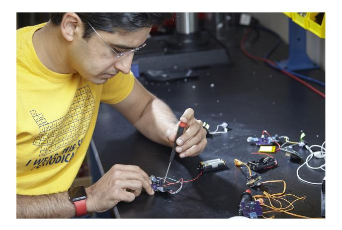
Georgia Tech assistant professor M. Saad Bhamla assembles a prototype LoCHAid, an ultra-low-cost hearing aid built with a 3D-printed case and components that cost less than a dollar. Credit: Craig Bromley
