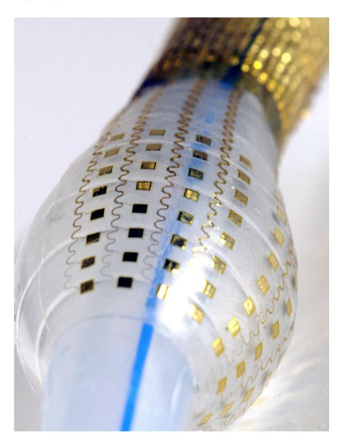
Seen here, a conformal array of electrodes affixed to an inflated balloon
