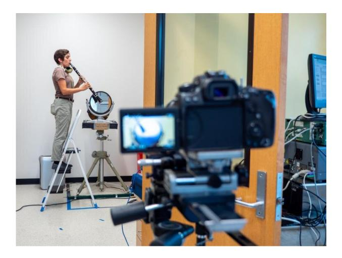
Stockman uses a DSLR camera to tape her clarinet performance to test for aerosol movement and dispersion from her instrument using a method called the Schlieren technique, in Miller's mechanical engineering laboratory on the CU Boulder campus. Credit: Glenn Asakawa/University of Colorado
