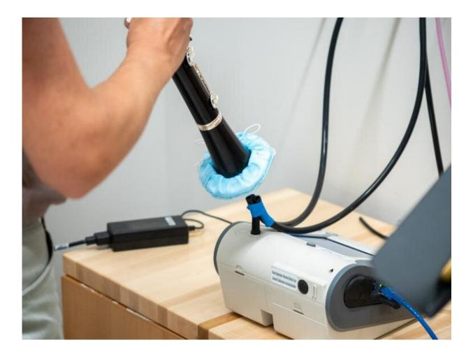
Teyha Stockman demonstrates how she plays her clarinet to test for aerosol particulate expulsion from the bell of the instrument. Stockman has fitted a homemade bell cover made from medical mask material to test for the effectiveness of lowering aerosol. Credit: Glenn Asakawa/University of Colorado
