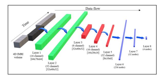
The simple yet effective architecture of the proposed CNN was carefully designed to handle 4D fMRI data through eight layers; the first two extract temporal features, the next three focus on spatial features, and the last three are geared toward classification. Credit: H. Parmar et al. doi 10.1117/1.JMI.7.5.056001.
