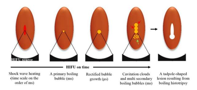
The mechanism and its shape of the secondary bubble generation. Credit: Korea Institue of Science and Technology(KIST)
