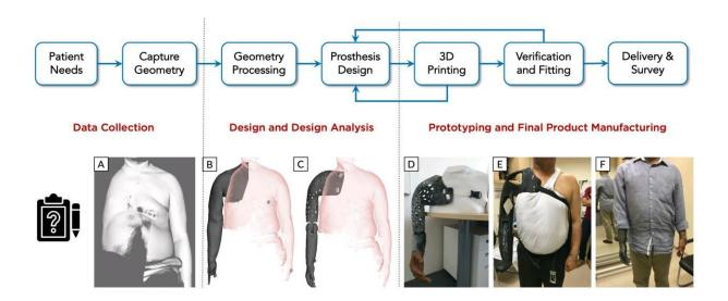
The schematic representation of the various stages involved in the user-centered, iterative process of prosthesis design. Credit: SUTD
