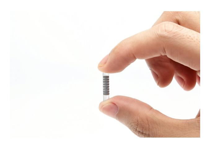
A flexible and biodegradable electronic blood vessel. Credit: Xingyu Jiang et al.
