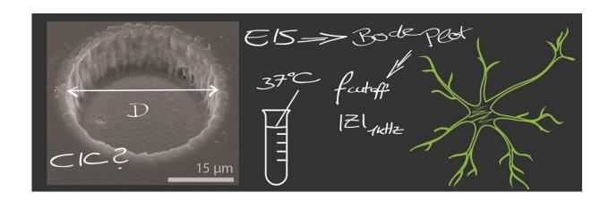
Analysis of characteristics of a microelectrode for receipt of electrical nerve cell signals at body temperature, photographed using a scanning electron microscope (left). Credit: Maria Asplund
