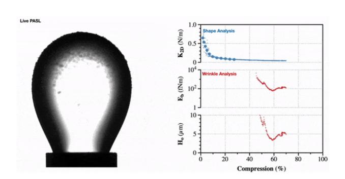
Researchers used pendant drop elastometry to compress and expand the biofilm that the PASL cells formed. Credit: Tagbo Niepa / University of Pittsburgh Swanson School of Engineering
