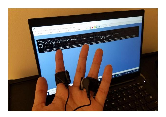
With electrodes strapped to two fingers, researchers can read out a signal of electrodermal activity. Credit: Sandya Subramanian/MIT Picower Institute
