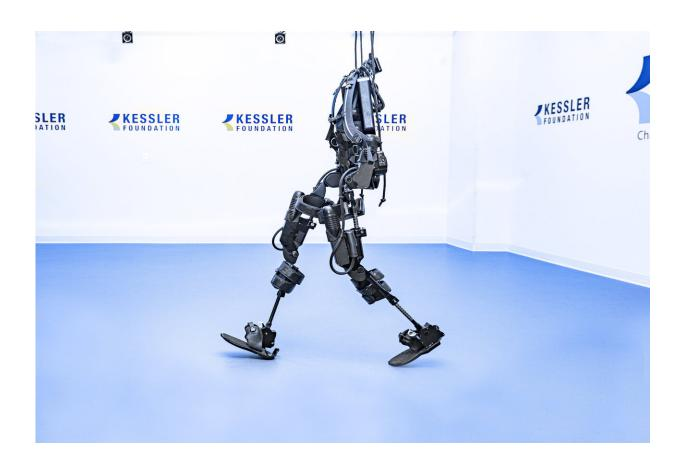
For this study, two types of exoskeletons were used by participants with spinal cord injury - Ekso GT, shown here, and Rewalk. Credit: Kessler Foundation
