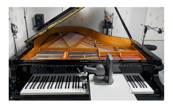
Haptic piano system. A haptic device (placed at the center in this picture) is attached to the piano. Credit: Masato Hirano
