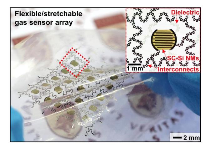
Flexible materials give researchers a chance to design sensors that are ideally suited for monitoring NO-type gases inside and outside of the body. Credit: Penn State
