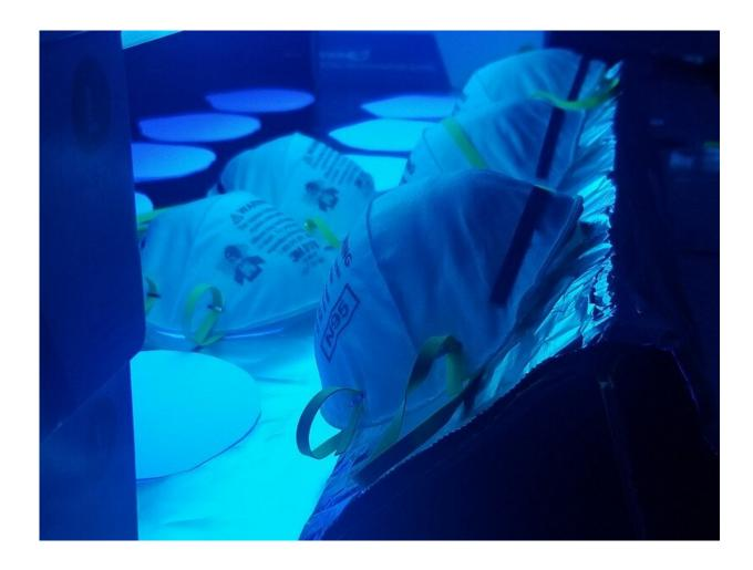
The UD research team created a sloped surface to help align masks situated along the edge of the system toward the light source for more uniform decontamination across the surface. Credit: University of Delaware
