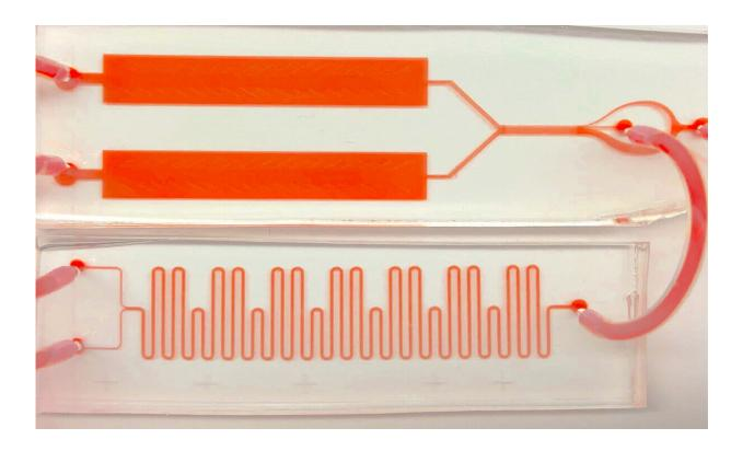
The RT-ELISA prototype consists of three modules: in the first (bottom), blood from the subject is mixed with a solution containing beads of target proteindetecting probes and fluorescent detection antibodies. The second module (topright) eliminates excess blood cells. And the third module (top-left), transfers the fluorescently labeled beads to a detection window for measurement by a highspeed camera. Credit: Caitlin Maikawa
